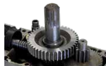
full metallic gearbox with 3-shapes of reduction
