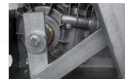
Easy maintenance thanks to the double greasers both on housing and gear motor
