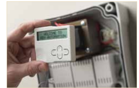
Control unit in box for two 24Vdc motors
